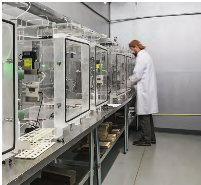
Small chamber formaldehyde testing at Benchmark International. (Photo by Alex Rhodes)
