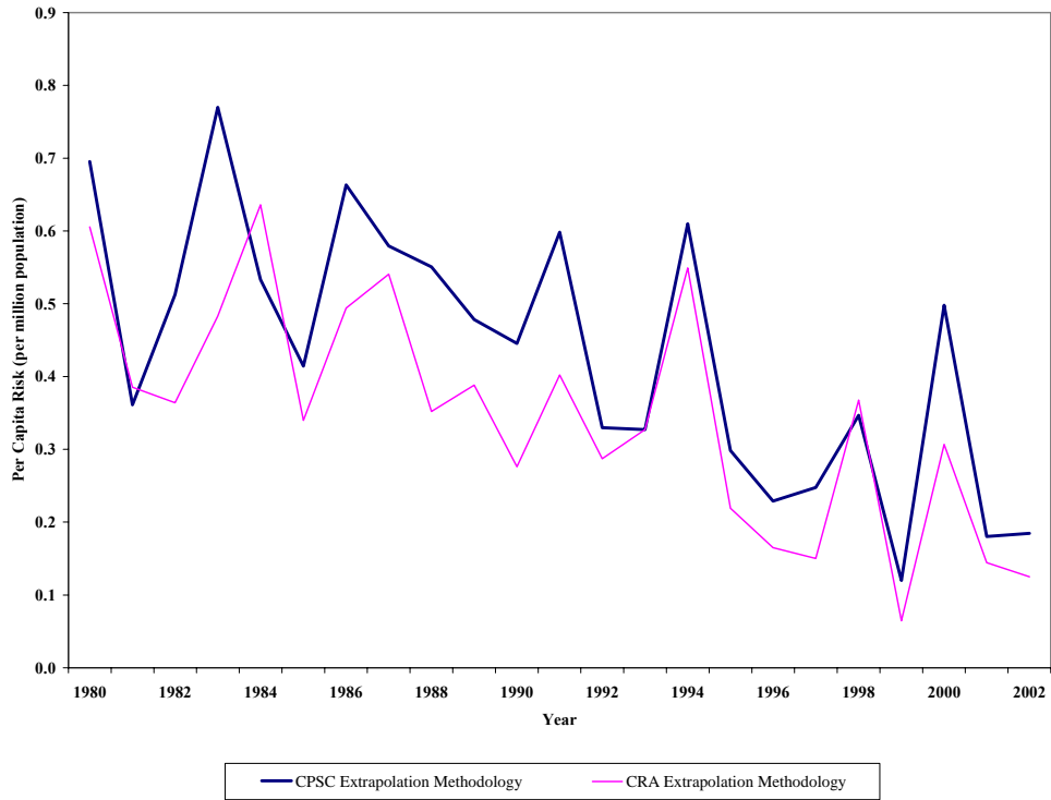
Figure 2b: Per Capita Risk of Death in a Small Open Flame-Ignited Furniture Fire, 1980-2002 (CPSC Extrapolation Methodology and CRA Extrapolation Methodology)
