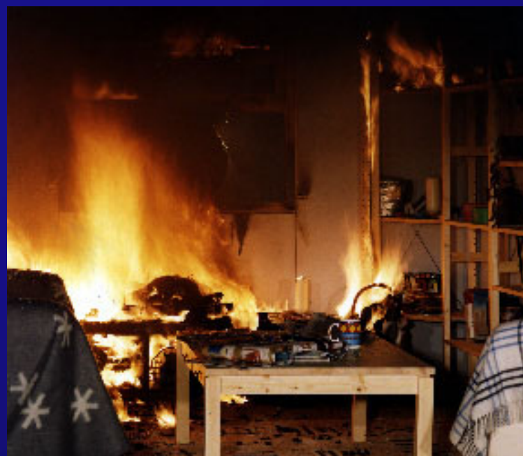
Room Fire: flashover 3 min 10 sec after starting a fire on sofa
